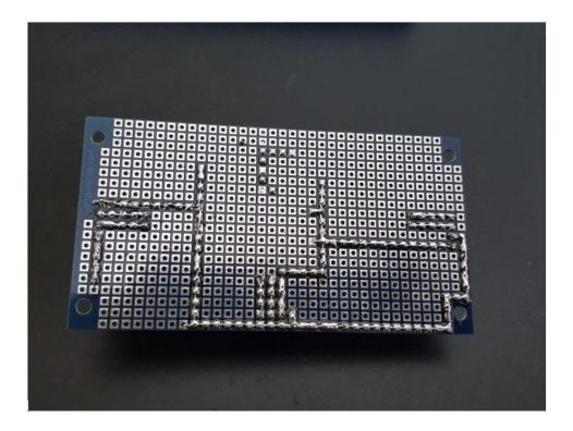
Unfortunately, we couldn't get a board for this PCB printed in time. The two images above is the circuit built onto a protoboard with solder bridges, while continuing to fulfill the requirements.
