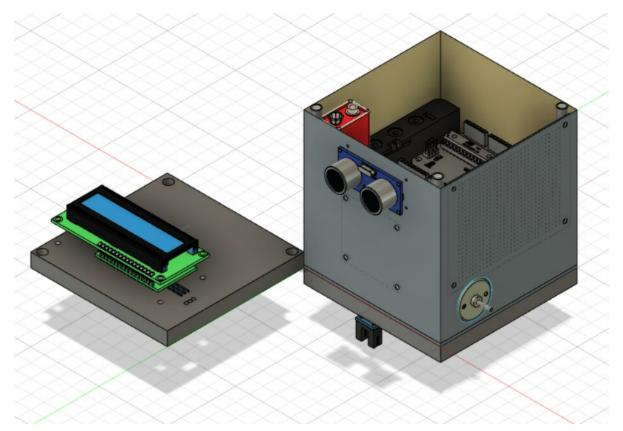
In the figure above, it represents the basic idea behind the enclosure of the sumo robot. The sumo robot will be a 10cm by 10cm box, and within that box will be all of the elements used to make the robot run. The sumo robot will have the lid on top which is designed to mount on top of the box. The front of the sumo robot is the surface with the Ultrasonic sensor on it; therefore, the forward direction would be where that surface is facing.
