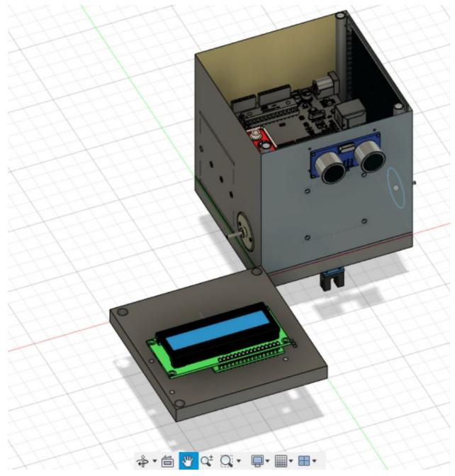
Finally, this last image shows a view where the PCB is present. On the far side of the sumo robot, the PCB that we created will be mounted onto the enclosure. Overall, that is the 3D model of the sumo robot. This 3D model can also be found here at this
