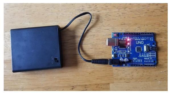
In the image above, it represents the schematic of the power source. Because our robot will be moving and be running for at least 15 mins, we will need a power source that is mobile. The figure above shows how we will be connecting a battery holder to the arduino using its power plugging port. Inside the battery holder are 4 AA batteries, and these batteries will be powering our whole sumo robot.
