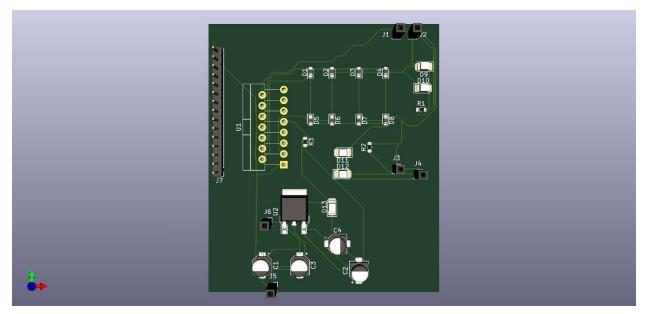
In the image above, the PCB is represented as a 3D model. On the left side of the board, the 15 pins will be aligned to fit into the arduino inputs. Then the rest of the circuit represents the dual H-Bridge layout. Then the circuit will connect to the motors and a power supply that will supply the motors.
