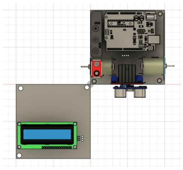
This image above is the 3D model at a view from the top. As we can see the mounting of the lid will be done by adding screws to the holes and directly into the columns that are in the same positions as the holes. We can also see that the LCD display has three holes next to it. Those holes will be used to let the wires through the enclosure and connected to the rest of the circuit. The sensors also have similar holes for the same reason.
