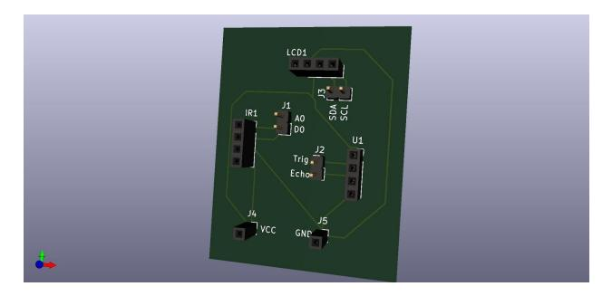
The PCB schematic and layout for the sensors and LCD display was created on KiCAD. The first image is of the layout, which shows the copper traces, pins, and board edges. The board itself measures 33.02 x 41.91 mm, or 1.3 x 1.65 inches. This is one of the simpler boards to make, since the sensors and the LCD display are already modules. The only thing that needed to be connected was the power and ground. The second image is a 3D rendering is what the PCB should've looked like.
