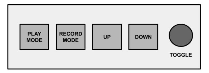
**Power On/Off:** Press and hold Toggle knob for 0.5 seconds. Melody Storm is set to PLAY mode when powered on.
