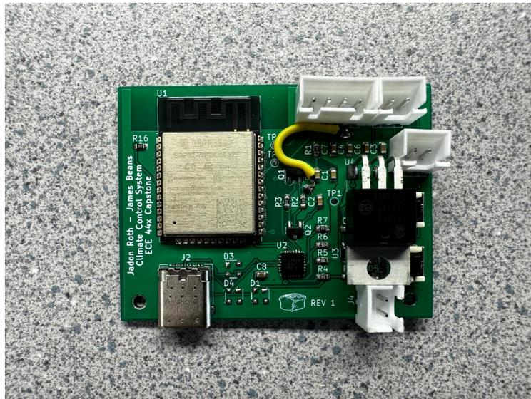
**Figure 5.3: Fully Assembled PCB**
