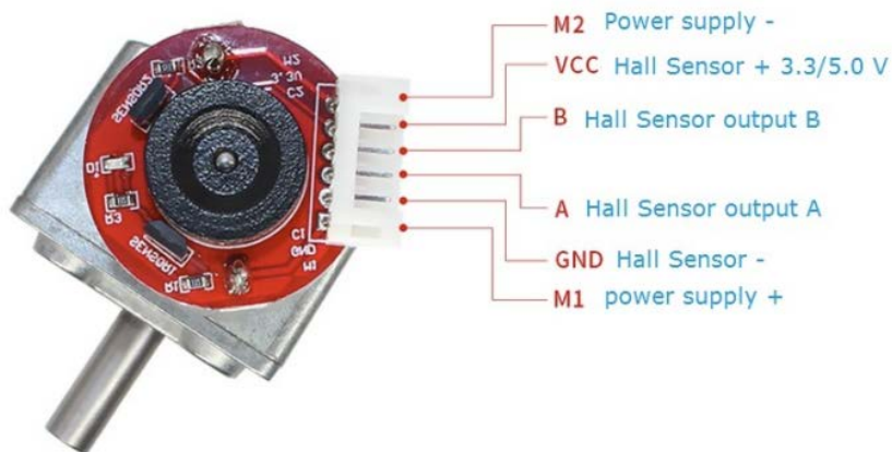
Figure 4.8.2: Motor schematic
