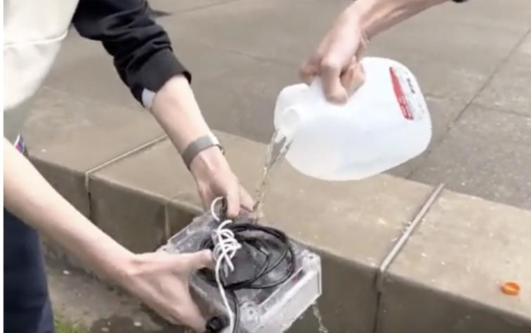
Figure 5.2.7.5: Weather Resistance Test
