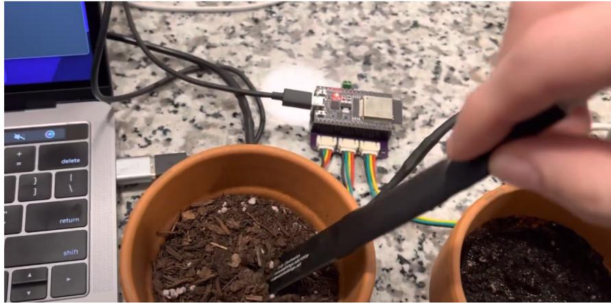
Figure 5.2.4.5: Soil moisture verification
