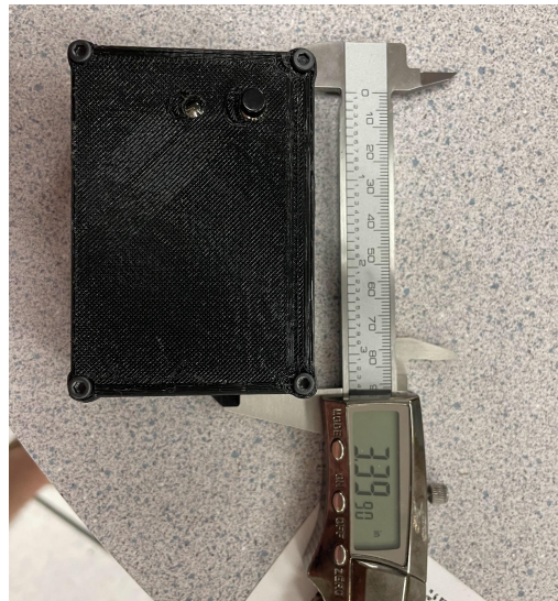
Figure 5.2.2.6.1: This image shows the length measurement of the enclosure.
