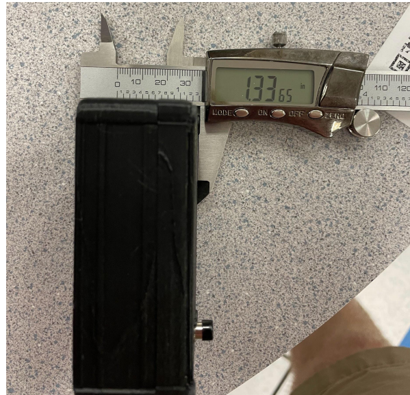
Figure 5.2.2.6.3: This image shows the height measurement of the enclosure.
