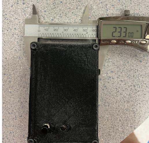
Figure 5.2.2.6.2: This image shows the width measurement of the enclosure.
