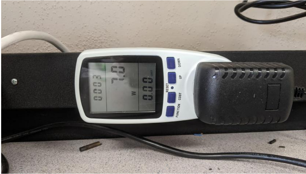
Figure 5.14: Joulemeter Setup for Efficiency Test
