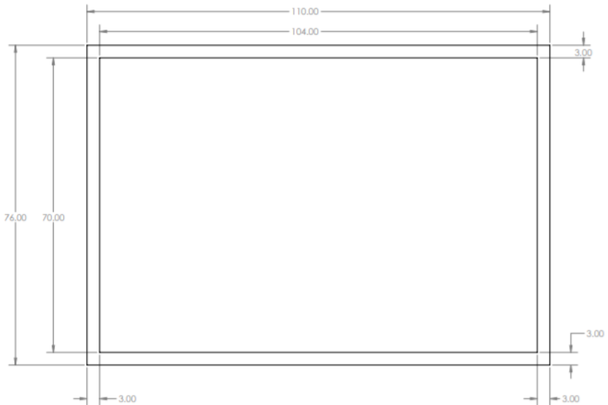
Figure 16: Bottom of enclosure lid
