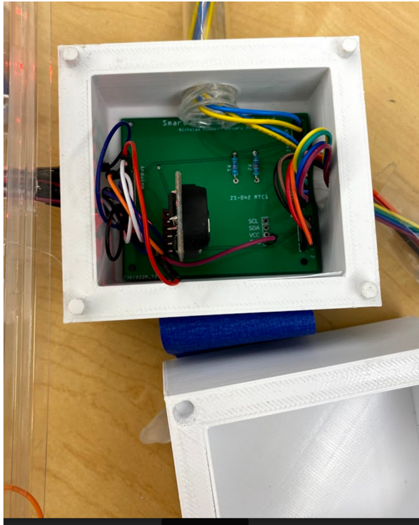
Photo of fully connected PCB in its enclosure with lid removed.
