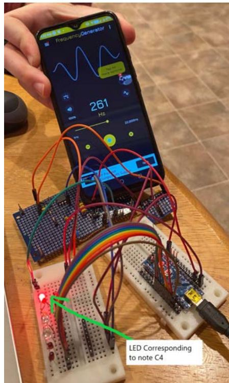
Figure 22: Validation of the LED circuit function with a note of C4.
