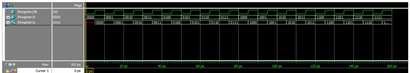
Figure 10.6.2: Derived waveforms from executing the do file above.
