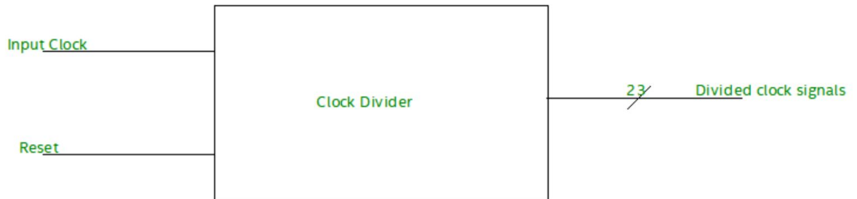
Figure 6.1: Block diagram of the Clock Divider module used.
