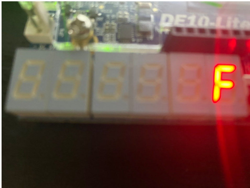
Figure 12.1: Seven segment output 'F'
