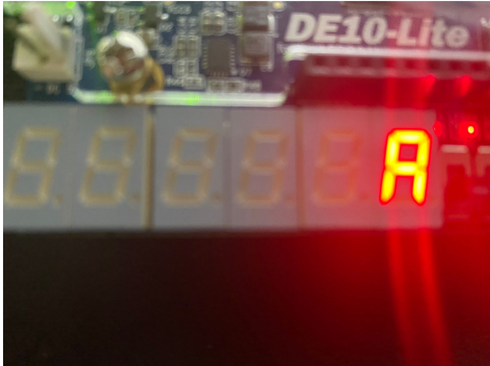
Figure 12.1: Seven segment output 'A'
