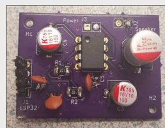
This PCB rests on the Control PCB and uses a LM386 audio amplifier to amplify signals sent from the microcontroller that drive the speaker.
