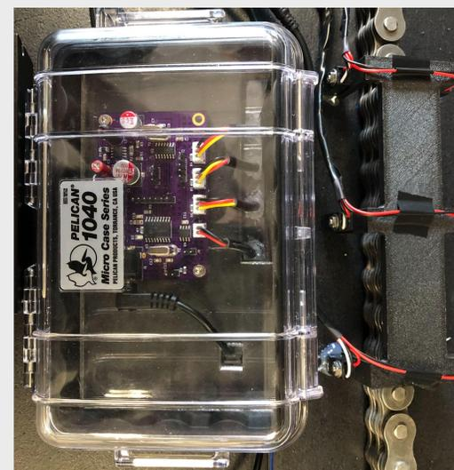
Fig. 3. Sensors bracket and PCB enclosure
