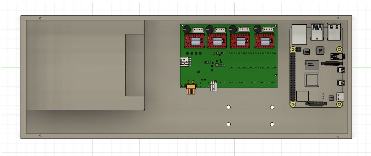
Figure 2: Enclosure with PCB, Power Supply and Raspberry Pi 4
