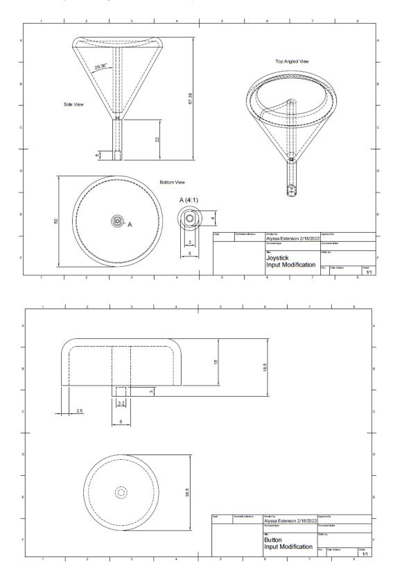
Mechanical Drawing for the Input Modification (Joystick and Button):
