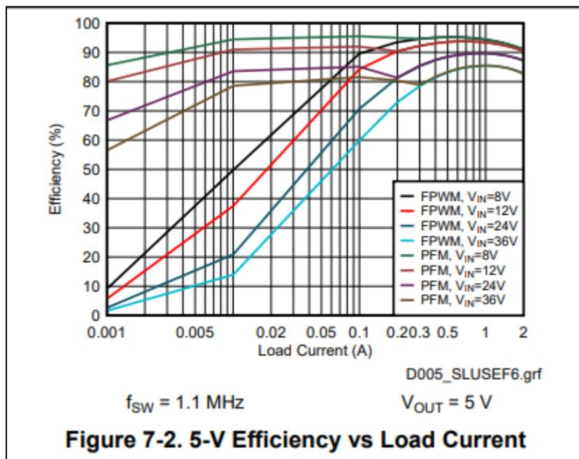
Figure 7-2. 5-V Efficiency vs Load Current
