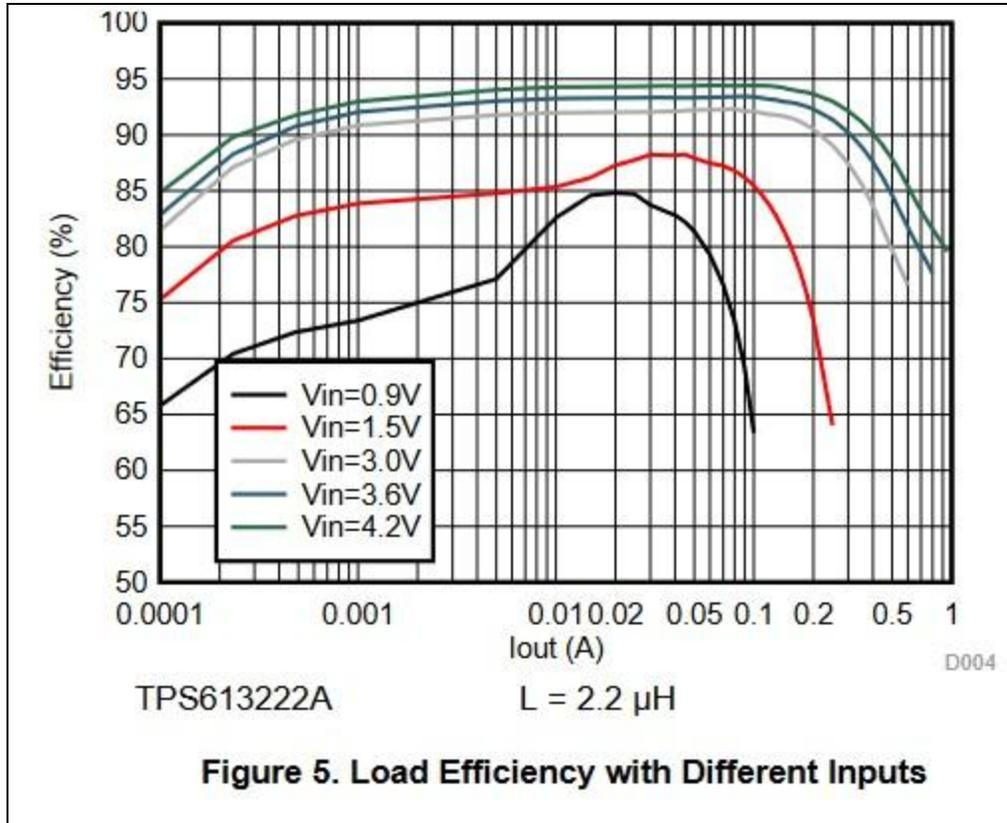
Fig. 5.1.4.2 - Efficiency of the TPS61322 boost converter pulled from the [datasheet](#). With an input voltage of 3.6V drawing 100mA of current the efficiency is approximately 93%.
