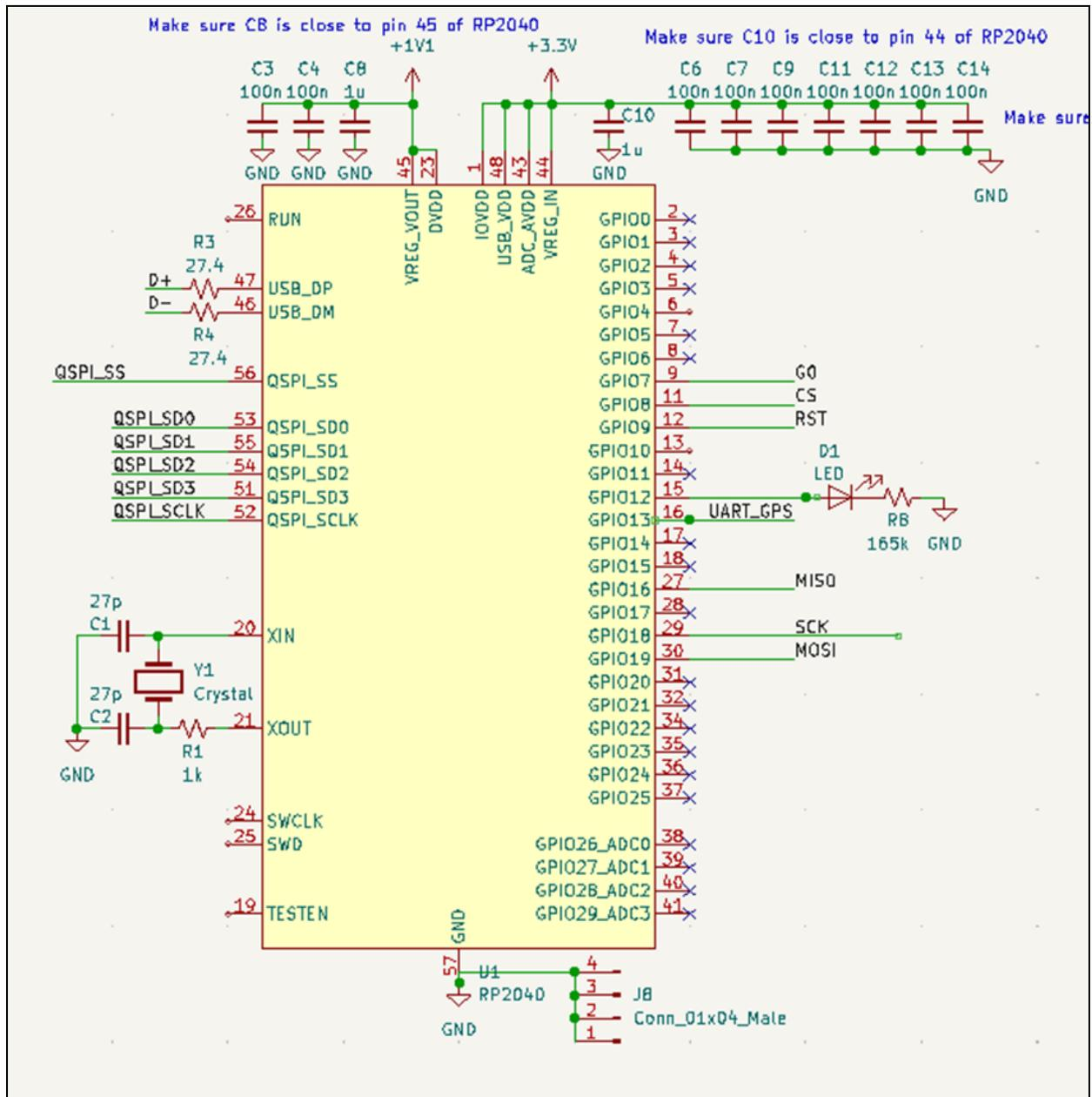
Fig. 4.3.2.2 - RP2040 is shown with connections to the GPS module and LoRa submodule, flash memory submodule, and the clock.
