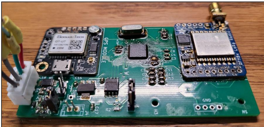
Fig. 5.1.1.2 - Universal Transceiver Board
