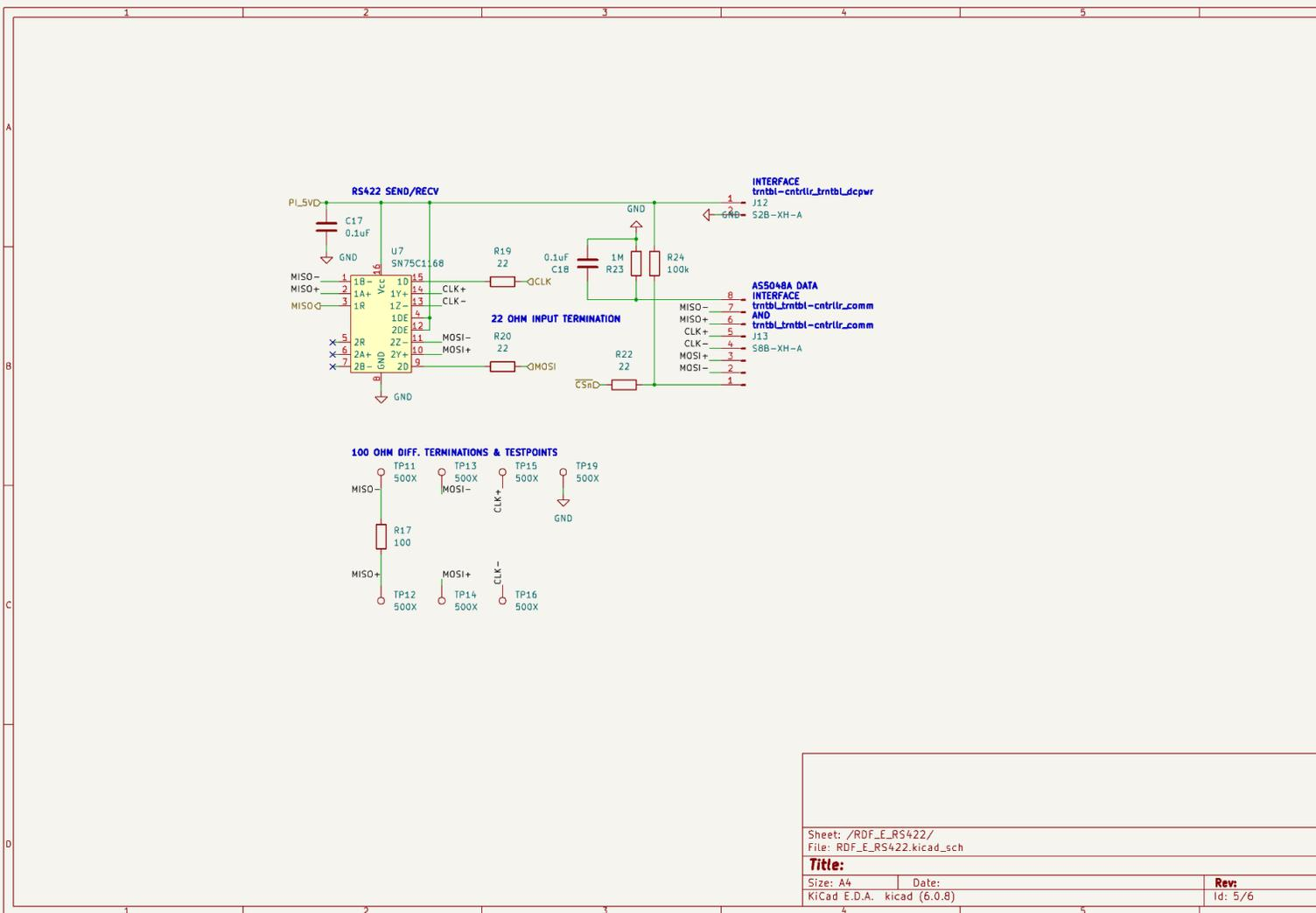
Fig. 4.5.2.4 - RS422 Sub-Circuit Schematic
