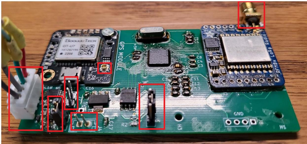
Fig. 5.1.3.1 - Transmitter PCB showing 7 connectors.
