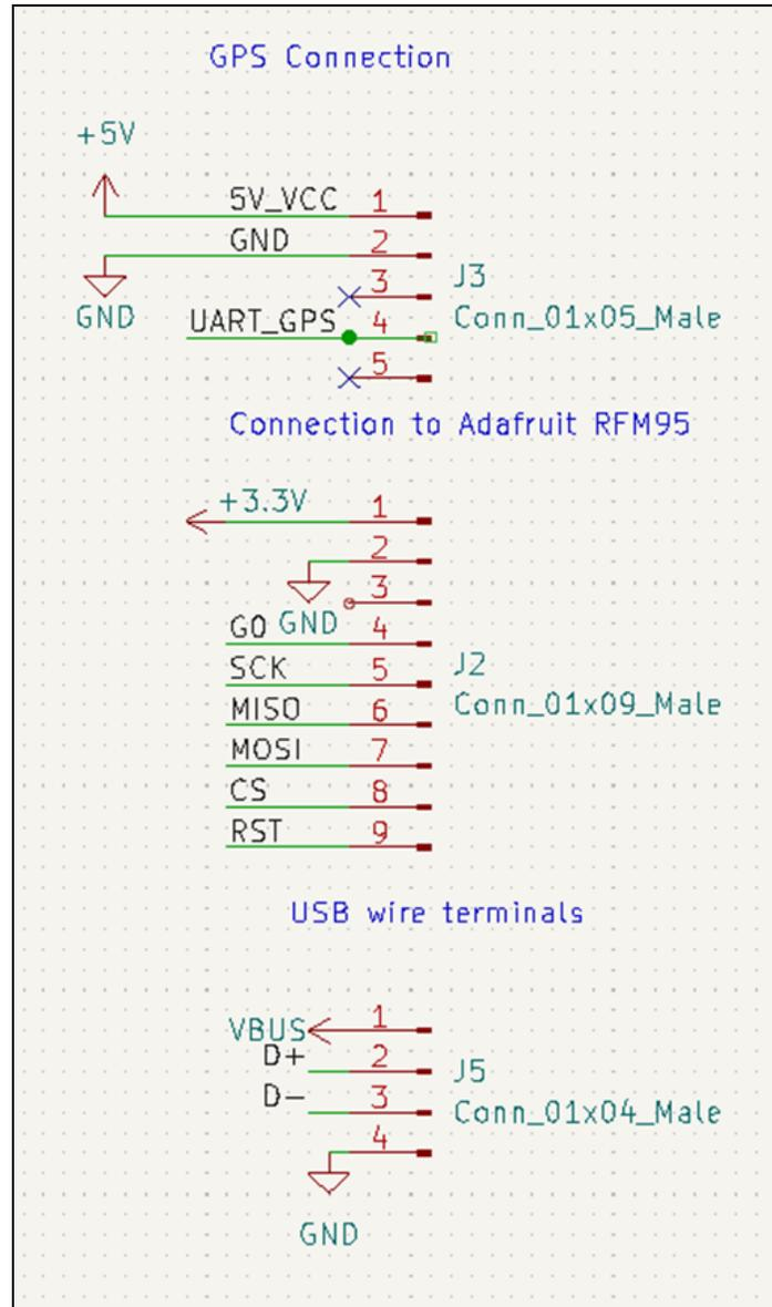
Fig. 4.3.2.5 - Pin connections for external sub-modules and USB
