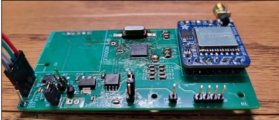
Fig. 5.1.2.3 - Transceiver implemented as a receiver
