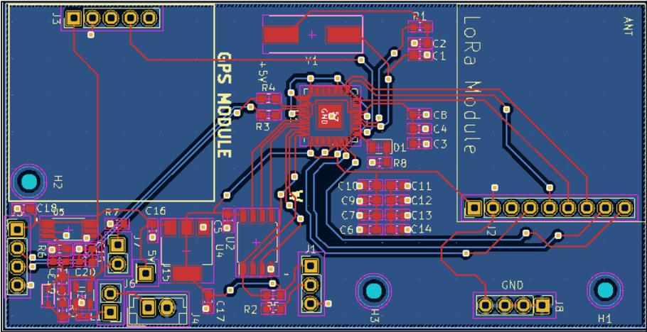
Fig. 5.1.2.1 - Transceiver PCB Design
