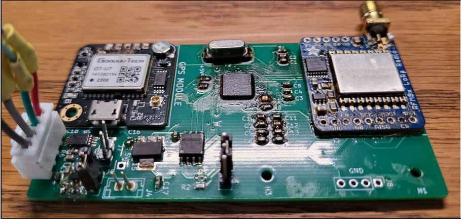
Fig. 5.1.2.2 - Transceiver implemented as a transmitter
