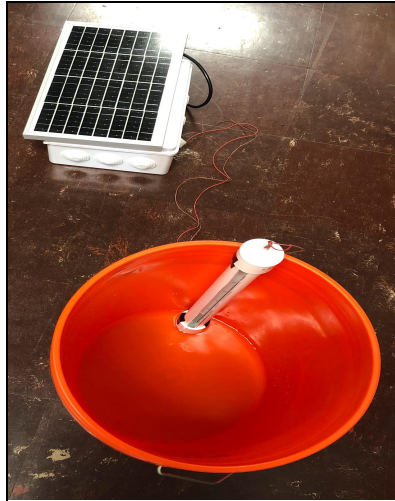
Figure 5.2-10: Water level setup for 0 inches of water.
