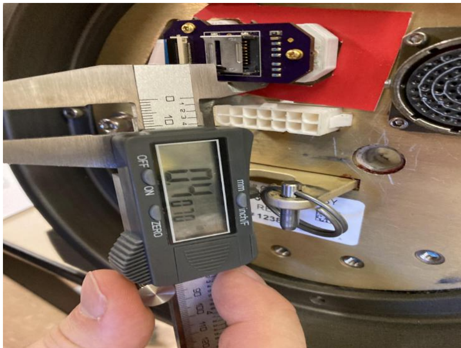
Figure 5.6.3.4: Demonstrating that the clearance requirement between the bottom white snap connector and the 3D printed bracket is greater than the required minimum of 0.25 inches.
