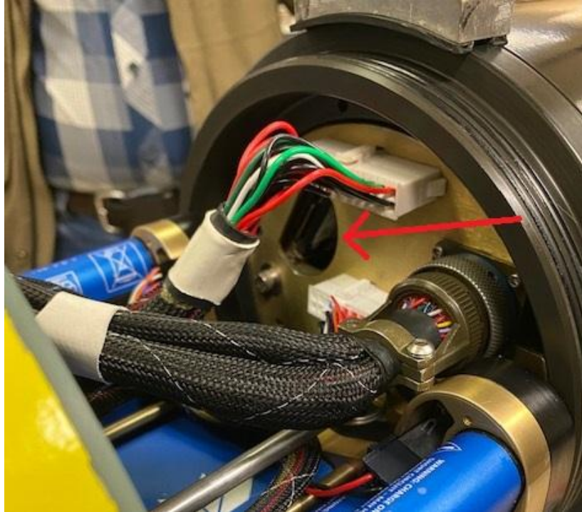
Figure 2.1: SD card retrieval hole in glider science bay.
