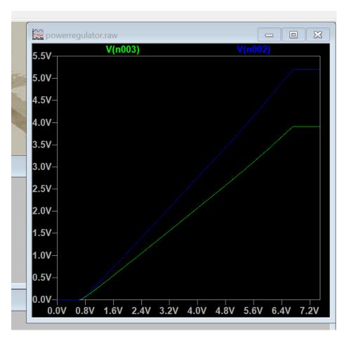
From the simulation, we could see that the output voltage is around 5V.
