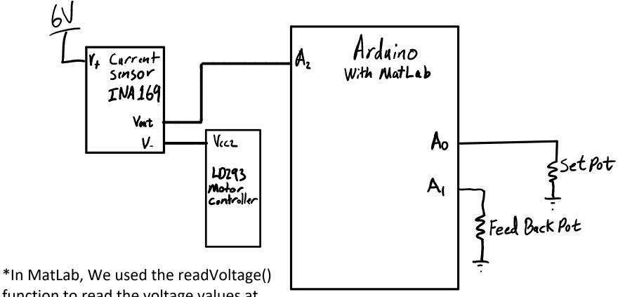
function to read the voltage values at A0, A1, and A2. There Voltages were used to create our plots.
