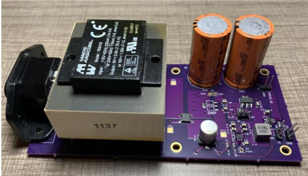
Figure 6.10: Power Supply Board Populated PCB
