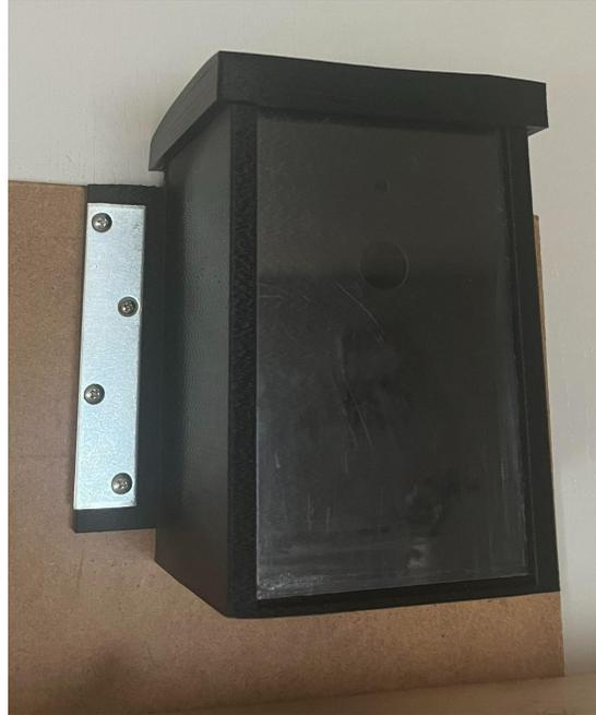
Figure 6.24: Printed Enclosure Assembled
