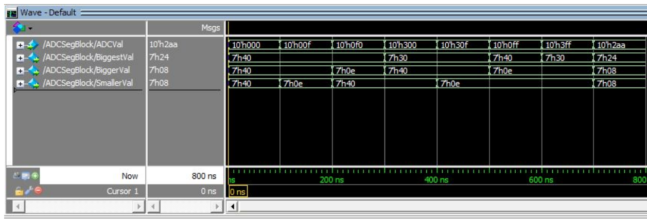
Figure 40: 7 segment display splitting 10-bit value into the separate digits.
