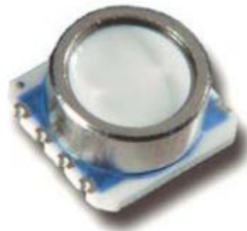
Figure x: The MS5803-02BA Pressure sensor being used
