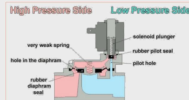
Figure 4: Solenoid-Controlled Valve mechanism example.
