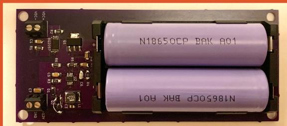
Figure 1: Custom Designed Solar Charging Boost PCB
